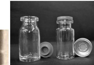
Figure 4-2 Glass vials with rubber closures and aluminum seal.
